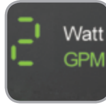
Large display shows estimated flow in gallons per minute
